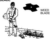
**NOTE:** Remove the trimmer head and plastic shield before attaching the metal shield and installing the weed blade. To remove the trimmer head, align hole in the dust cup with the hole
